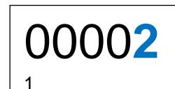
Press the S key to save the operation code. The bottom left side of the display will show the operation code 2 to indicate enter the function "Unit Settings."
