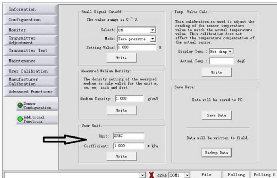
In the "User Unit" box, indicated by the arrow in the previous figure, write the user unit you want to use. Enter the value of the "Coefficient", which must always be the maximum value of the calibration range divided by the maximum value of the user unit range.
